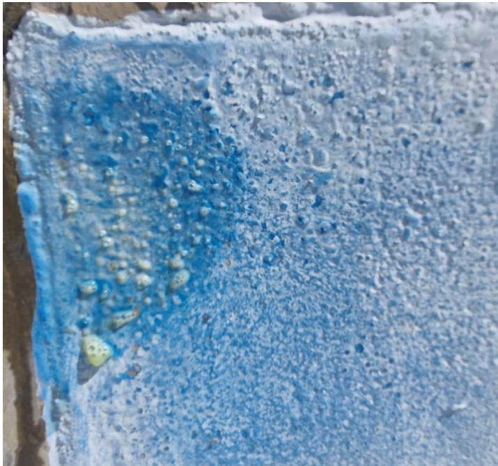
Fig 4. The results of neat HCL (Pool Acid) on the white material and the fizz indicate its \text{CaCO}_3 the result. The paint in this case is unaffected by the pool acid. There are usually other salts there also, and some of these also react with the pool acid.
