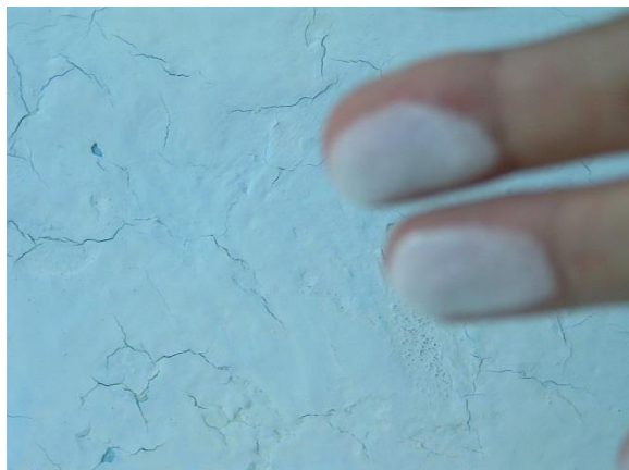
Fig 1: Paint can become chalky over time and leaves a film on your figures. This happens sooner with Chlorinated Rubber (1 – 2 yrs) and takes much longer with Epoxies. (5 -8 yrs) and for a MUCH longer life, Fluoropolymer, which does not chalk. It may also be quite often the result of insoluble residues in your (especially salt) pool. Need to check which.
