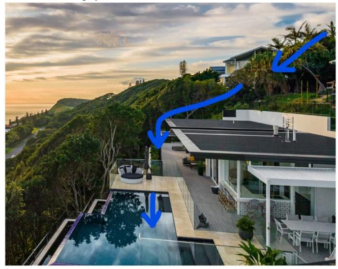
An example of a pool close to a home and potential cool air flowing down hill and into the pool.
