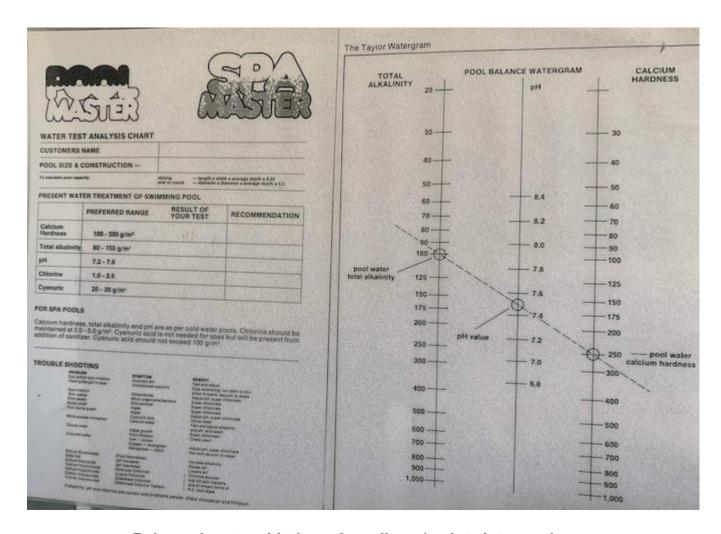
Balanced water with these 3 readings / points intersecting
